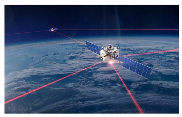
FSO (**F**ree **S**pace **O**ptic) is a line-of-sight technology that uses invisible beams of light to provide optical Bandwidth Connections capable of sending up to 1.25 Gbps full duplex of voice, video, and data information's.
